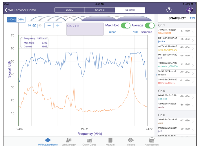
Spectral view shows interference within a channel
