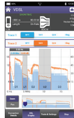
Bits-per-tone (BPT) vs SNR graph
