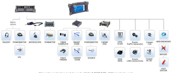
Fiber optics application modules used with the T-BERD/MTS-4000 can also be used with the T-BERD/MTS-2000 and the two products are interoperable
