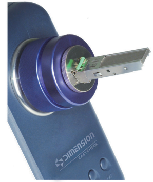
LC Transceiver Inspection
