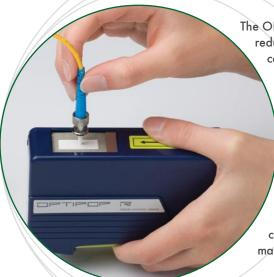
The OPTIPOP R is a cassette style fiber optic connector cleaner system that can be refilled for reducing cleaning costs. It uses a densely woven micro-fiber cleaning fabric to remove harmful contaminates off of the ferrule end face. The OPTIPOP R cassette cleaning tool will
