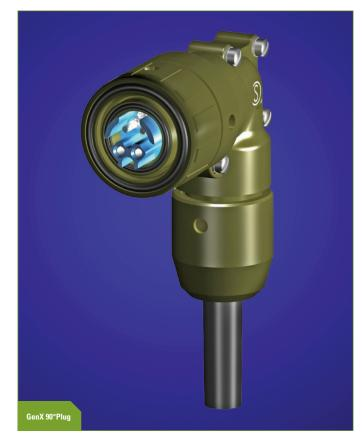
STRAN's TFOCA GenX<sup>™</sup> 90° Plug Connector is designed for mounting applications where the installer has limited workspace or the connection needs to be re-routed close to equipment. One major advantage of this connector is its short length of 3.20″ making it ideal for cabinet or equipment mounted fiber connections.
