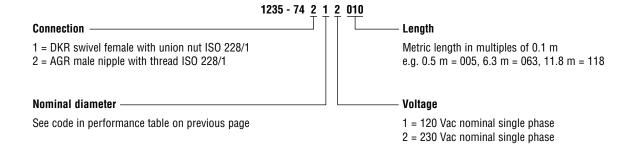
**Example:** 1 m heated hose, 4 mm nominal diameter, 230 V supply voltage, AGR connection
