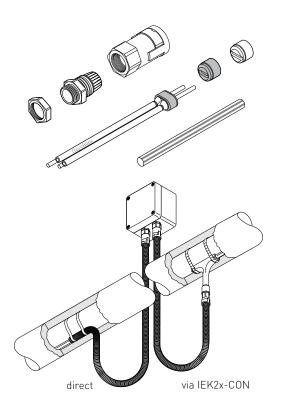
This connection kit is designed for terminating all Raychem BTV, QTVR, XTV, KTV and VPL parallel industrial heating cables to a junction box, whilst maintaining electrical insulation of the heating cable conductors and core as well as providing a reliable and sealed connection to a conduit system. It is approved for use in hazardous locations.
