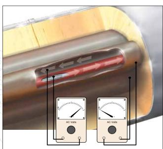
AC voltage will generate a current in the conductor which returns through the inside surface of the heat tube. There is virtually no measurable voltage on the outer surface of the heat tube, allowing the piping system to be grounded.
