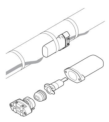
The E-150 is a cold applied low profile end seal. This universal end seal is designed to fit with all Raychem industrial self-regulating heating cables; BTV, QTVR, XTV and KTV meaning simplified product selection and reduced inventory to stock. It can be used in applications with temperatures ranging from -50°C to 215°C. It is approved for use in hazardous areas.
