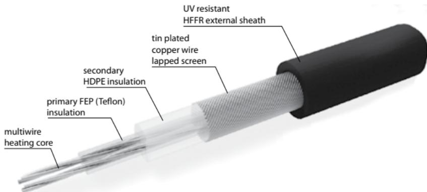
ELEKTRA SnowTec®<sub>Tuff</sub> heating mat's cable structure
