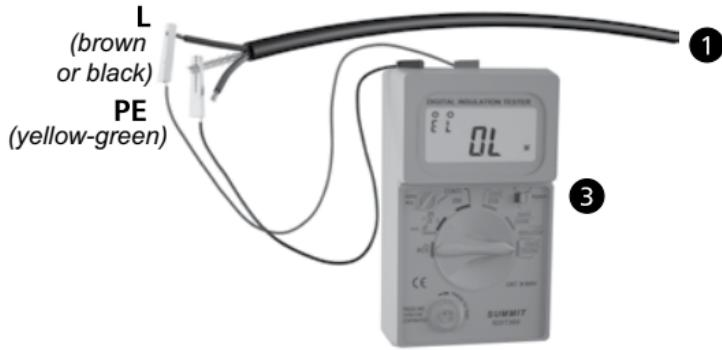
Insulation resistance measurement
