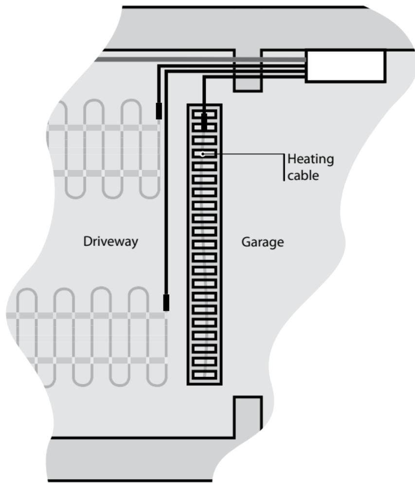
Linear drainage heating
