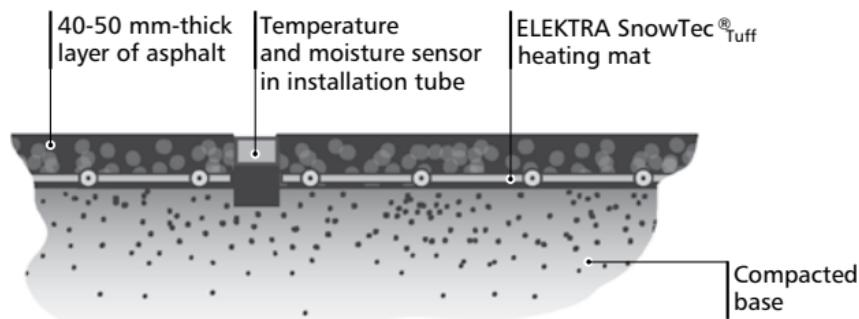
Cross section of a driveway or road with asphalt surface
