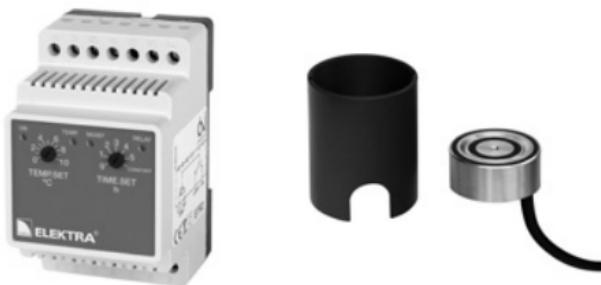
ELEKTRA ETR2G controller – max. load up to 16 A, total output of installed heating cables must not exceed 3600 W. As standard, equipped with one temperature and moisture sensor with installation tube.
