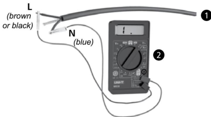
Heating wire's resistance measurement
