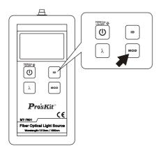
After pressing " button, you can load a confirmed carrier frequency in the current output laser.
