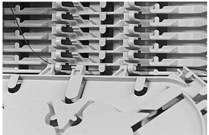
5.2.5 Route the fibers in the grooves of the wraparound groove plate to the entrance of the identified tray. Fiber must be routed in the groove underneath the tray hinge.
