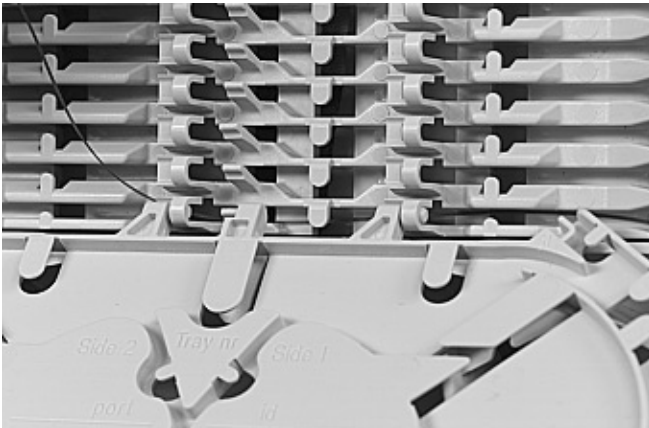
4.3.6 Route the fibers in the grooves of the wraparound groove plate to the entrance of the identified tray. Fiber must be routed in the groove of the tray hinge.
