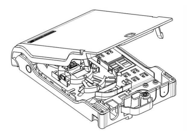
**OptiBox 4** is a fiber optic distribution and termination enclosure, which is used for splicing, patching and to perform with passive optical components.
