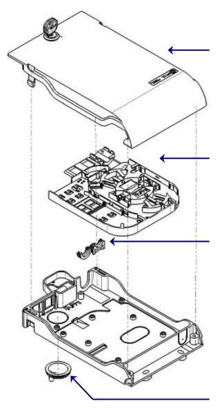
1 clip- on cover equipped with a key lock: cylinder quarter trun lock model with spring fixing protected access to lock fixation cover is individually lead sealable
