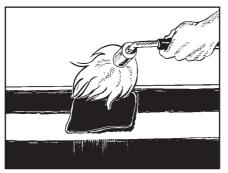
2. Position the precut PERP patch over the damaged area and heat until the adhesive melts. Roll out any entrapped air with a silicone roller.
