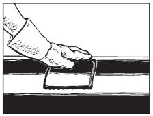
4. Smooth the repair patch with a gloved hand to eliminate air entrapments and ensure good bonding. Avoid squeezing filler between PERP and the line coating.
