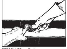
**PERPFILLER** application 1. Cut PERPFILLER to size and apply it to all areas of exposed steel.
