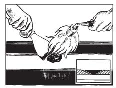
2. Heat the mastic and smooth it down with a paint scraper to cover all bare metal without air entrapments. Avoid traces of PERPFILLER on top of the PE coating.
