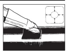
3. Cut a patch from the PERP tape so that it extends at least 50 mm (2") beyond the damaged area. Round off the corners.
