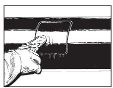
3. Check that adhesive is soft to the touch of a gloved finger.
