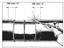
4. Grid or sand blast the adjacent pipe coating over a distance of at least 100 mm (4"). The total width should be approximately 50 mm (2") larger than the width of the supplied HTLP80 sleeve.
