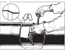
**9.** Immediately after preheating, apply the mixed epoxy primer to the bare steel using an approved application pad. Visually check the surface and ensure all bare steel is covered by the epoxy primer.
