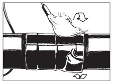
**17.** Continue heating towards the other end of the sleeve. Ensure that the total sleeve has been heated evenly and has completely shrunk tightly around the pipe.
