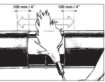
7. Adjust the torch to a yellow topped blue flame of approximately 500 mm (20") long. Preheat the steel and the adjacent pipe coating to 70° C (158°F) minimum, 90° C (194°F) maximum. Preheating of the surface reduces the installation time and ensures proper bonding.
