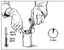
6. Dose the two component epoxy. Use pre-dosed epoxy kits or use calibrated epoxy pumps.
