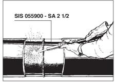
3. Grid blast or sand blast the steel surface to remove loose and foreign materials. The surface should be cleaned to SIS 055900 -SA 21/2.
