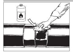
1. Clean exposed steel and adjacent pipe coating to be covered by HTLP80 sleeve. Remove all contaminants such as oil. Use a solvent that contains no grease or oil type materials.
