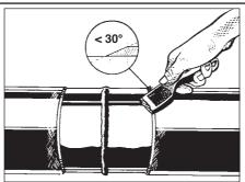
2. If not factory beveled, chamfer the adjacent pipe coating to an angle of preferably 15°, maximum 30°. Inspect the edge of the existing pipe coating. Disbonded sections have to be trimmed of and the coating edge has to be beveled again. To avoid possible contamination, it is recommended to use a scraper.
