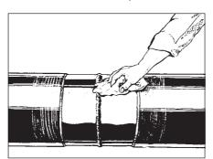
5. Wipe the surface to remove dust and remaining blasting material. Use a clean dry cloth or air blow.
