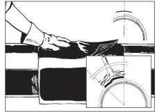
**13.** Heat the inside of the closure patch for 1 - 2 seconds. Position it evenly over the edge of the heat shrinkable sleeve. Press it down firmly.
