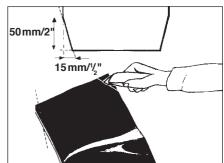
**10.** If not factory cut, cut the corners of the underlaying end of the sleeve to approximately 15 mm x 50 mm (1/2"x2").
