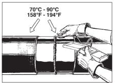
**8.** Check the preheating temperature with a contact pyrometer or a recommended temperature indicator strip.
