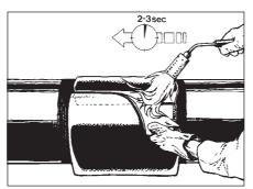
**12.** Gently heat the inside of the overlapping sleeve edge and press down onto the opposite sleeve and with a gloved hand.
