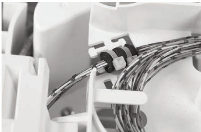
5.10 In case of pre-connectorized MINI PICO cable, fibers are also routed behind the tower and secured with foam and tie-wraps onto the tray.
