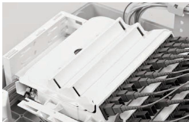
6.3 Install the cover onto the patch tray.
