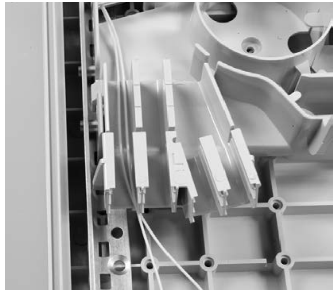
9.3 Route the pigtails towards the FAS block.
