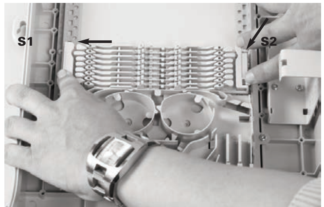
10.1 Secure the wraparound groove plate on the UMS by putting the plate with the long protrusions in the S1 UMS-profile and sliding the plate in the S2 UMS-profile until it snaps. (Do not leave gaps between groove plates).
