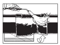
Start heating the sleeve at the side of the leading edge, the side that first comes in contact with the ground forces. Move the torch continuously in a paint brush motion all the way around the sleeve.
