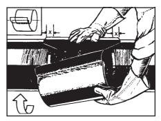
Immediately after application of the epoxy primer, and while the epoxy primer is still wet, loosely wrap the DIRAX sleeve centrally around the welded joint.
