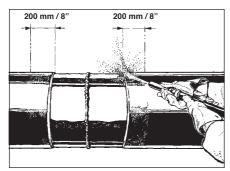
Grid or sand blast the adjacent pipe coating over a distance of at least 200 mm (8"). The total width should be approximately 50 mm larger than the width of the supplied DIRAX sleeve.
