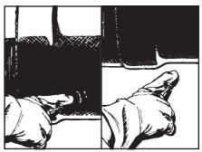
During shrink down, check adhesive flow with finger occasionally. Wrinkles should disappear automatically.
