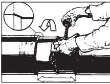
Using the supplied applicator pad, apply the mixed epoxy primer over the entire surface to be covered. (When PE line coating is used, no primer should be applied over the polyethylene line coating.)
