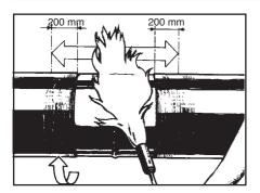
Preheat the bare steel surface and adjacent coating to minimum 70°C (160°F), using propane torches. Adjust flame length to approximately 20" (500 mm). In cold conditions extra heavy preheat torches can be used. Check preheat temperature with a contact pyrometer.
